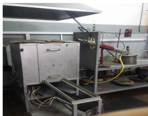
Fig. 2. Laboratory 5-kg electric coking furnace
