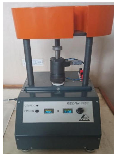
Fig. 1. Testing unit for determining the coke powder SER
