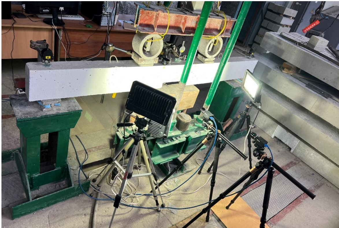
Fig. 7. Overall view of the camera arrangement for image capture.
