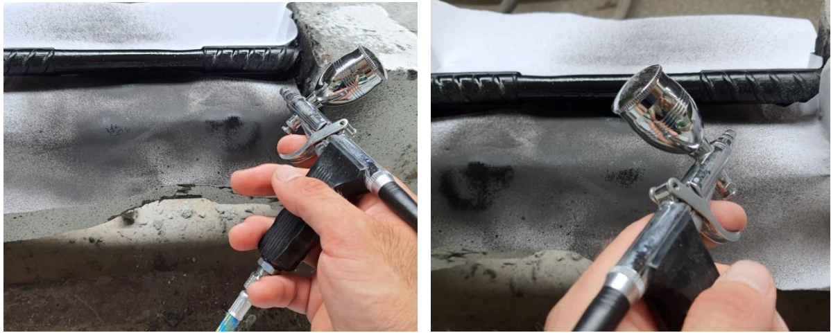
Fig. 3. Application of speckles on the reinforcement using an airbrush.
