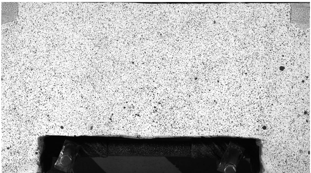
Fig. 5. Applied speckles on concrete.
