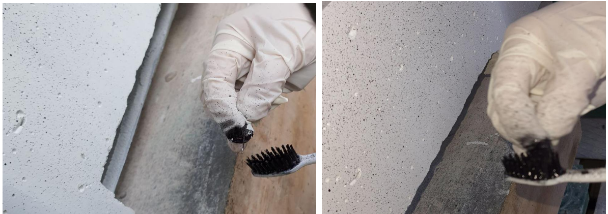
Fig. 4. Application of speckles on concrete using the spraying method.
