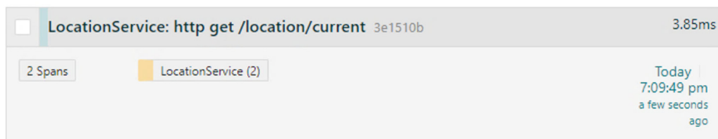
Fig. 18: Location service is invoked without parent context (API Gateway and Weather Service)
