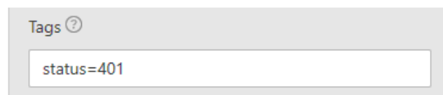
Fig. 12. Applying filter to see all unauthorized requests
