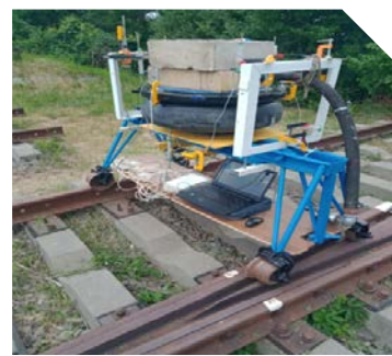
Movement of the test rig by the switch cross
