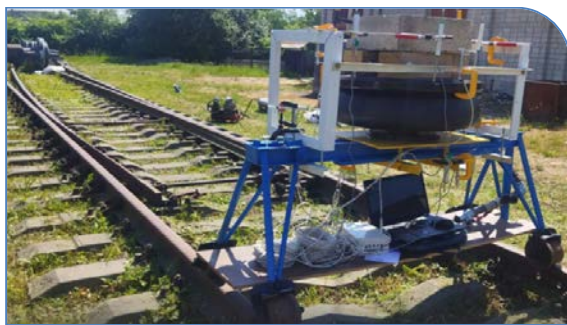
Movement of the test rig along the switch point
