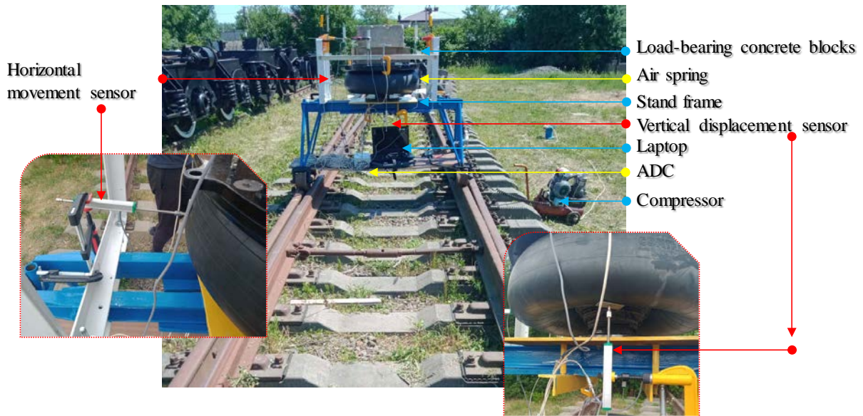
Fig. 5. Movable test rig for researching the lateral sway of the pneumatic spring of high-speed rolling stock
