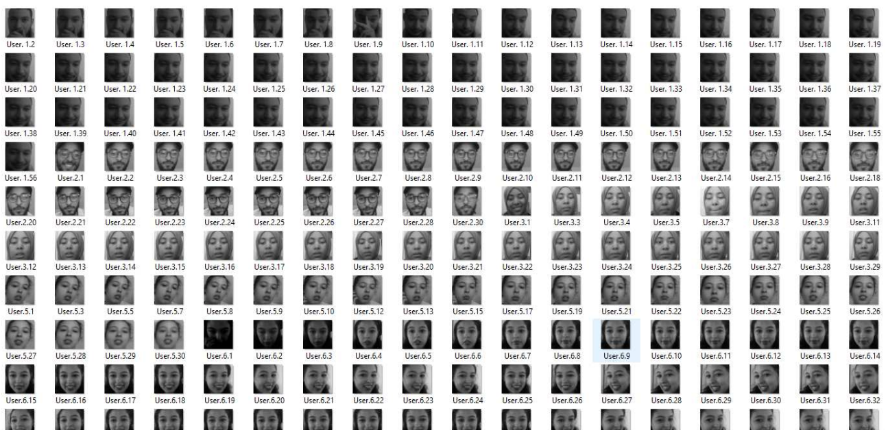
Fig. 4. Database preprocessing for facial recognition: grayscale conversion and normalization.
