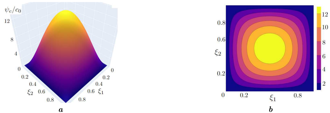
Fig. 10. Correlation function for the interval of action of the point source system [0.8, 0.9] at \tau_1 = 0.5 and \tau_2 = 0.45 .
