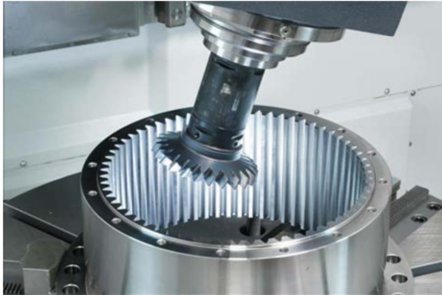
Fig. 1. General view of an internal gear machined by power skiving [5]
