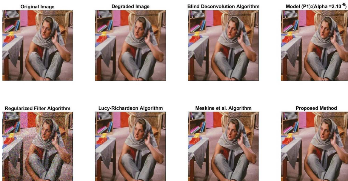
Fig. 3. Comparison of the proposed deconvolution model applied on a blurred Barbara image, with different existing methods: Meskine et al. model, Model (P1) ( \alpha = 2.10^{-6} ), Blind Deconvolution algorithm, Regularized Filter algorithm and Lucy–Richardson algorithm.
