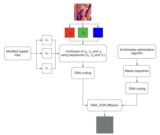
Fig. 3. Bloc diagram of the proposed encryption scheme.
