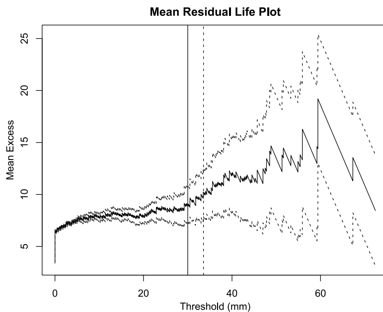
Fig. 2. An illustration of the MRL plot derived from daily rainfall data. The dashed line represents automated threshold selection approach. The solid line represents threshold value using the MRL plot technique.
