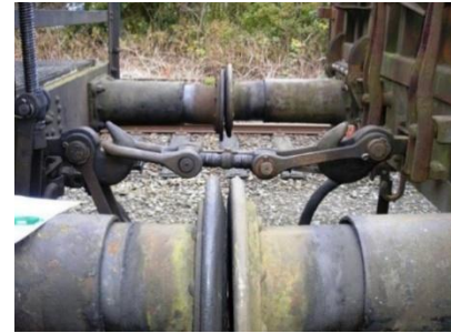
Fig. 1. General view of the screw coupling with buffer devices
