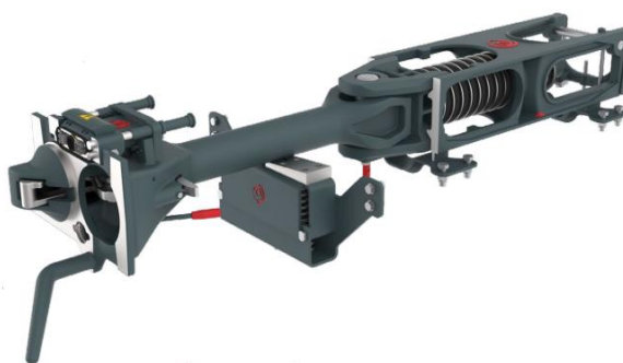
Fig. 5. General view of the Scharfenberg-type automatic coupler manufactured by Wabtec Corporation [12]
