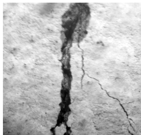
Fig. 2. Typical image of a concrete surface with a crack using camera has the resolution of 3280 \times 2464 pixels with a pixel size of 1.12 \mu\text{m} \times 1.12 \mu\text{m}
