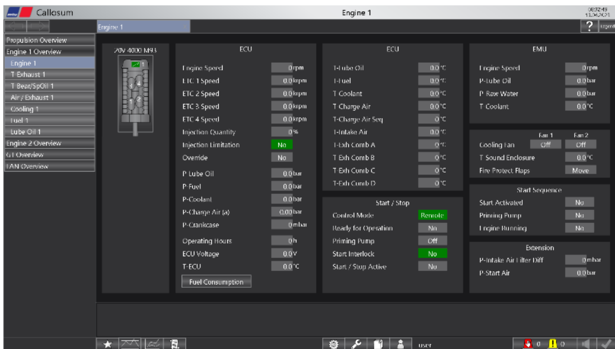
Fig. 2. Visualization of current values of determining parameters on the digital display panel.
