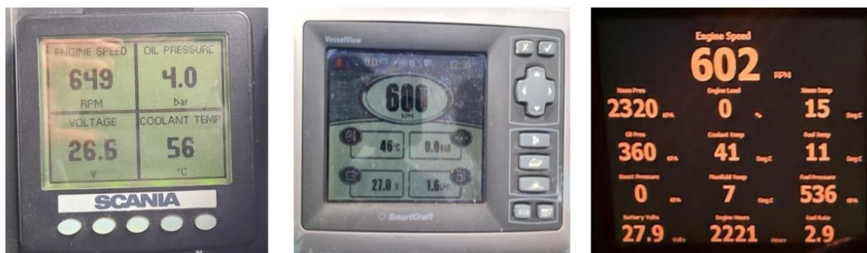
Fig. 3. Types of digital display panels of on-board instruments for controlling and monitoring the powerplant.
