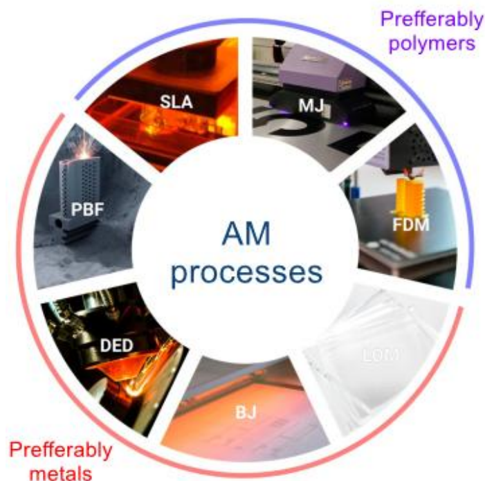
Fig. 1. Classification of additive manufacturing processes in accordance with ISO/ASTM 52900:2015. Material Extrusion (FDM and FFF), Photopolymerization (SLA and DLP), Powder Bed Fusion (PBF, SLS, DMLS, and SLM), Material Jetting (MJ), Binder Jetting (BJ), Directed Energy Deposition (DED), and Laminated Object Manufacturing (LOM) [8-12].
