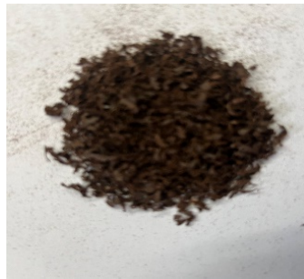
Fig. 3. Finely dispersed biomass of thermally modified ash wood exposed in the natural environment (TM-Ash 24 ) which was used to prepare biomass test samples (Biom-TM-Ash 24 )
