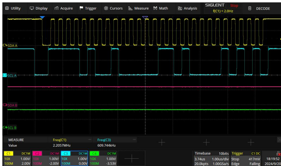
Fig. 5. I^2C Level shifter scope shot, 3.4 MHz frequency (outputs disable).
