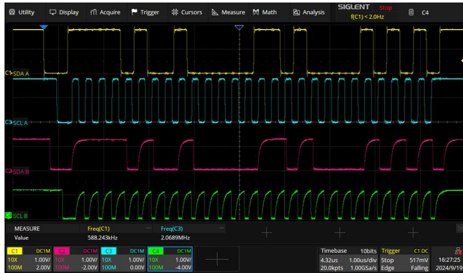
Fig. 3. I^2C Level shifter scope shot, 3.4 MHz frequency (A to B transition).
