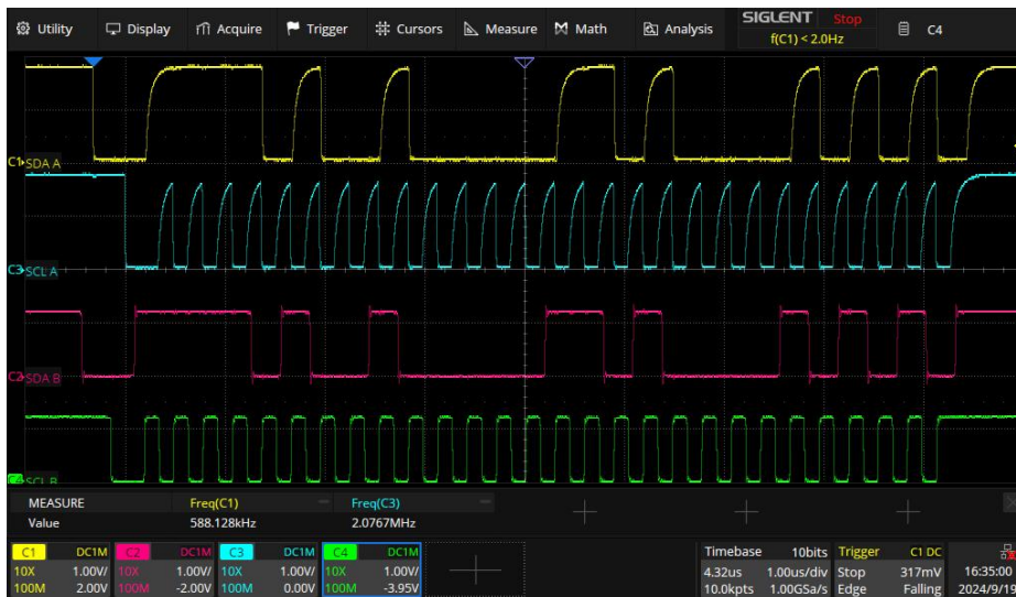
Fig. 4. I^2C Level shifter scope shot, 3.4 MHz frequency (B to A transition).
