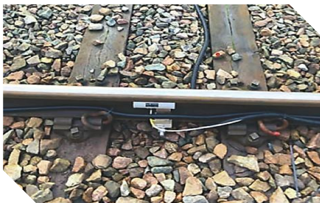
Fig. 1. Placement of acoustic sensors on the railway track, warning system for approaching rolling stock to a level crossing (LCWS) [13]
