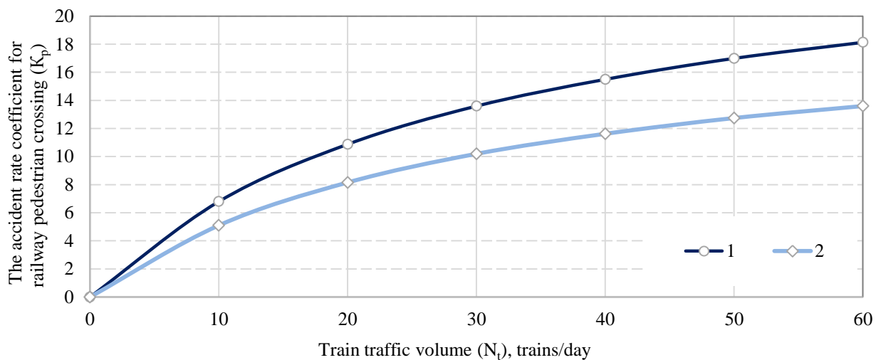
Fig. 2. Dependence of the accident rate coefficient at a railway pedestrian crossing on the number of trains per day: 1 – railway crossing without a pedestrian warning information system; 2 – railway crossing with a pedestrian warning information system.
