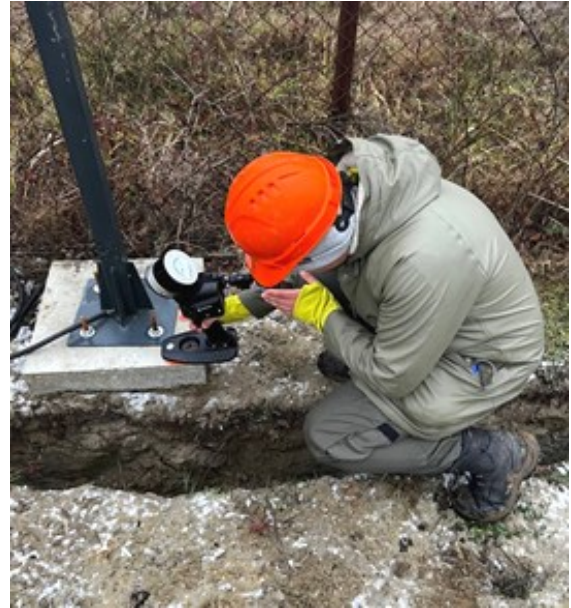
Fig. 6. Setting up the scanner on the control point
