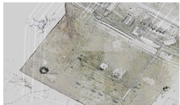
Fig. 19. View of an orthophotoplan fragment – adjusted point cloud density and display color
