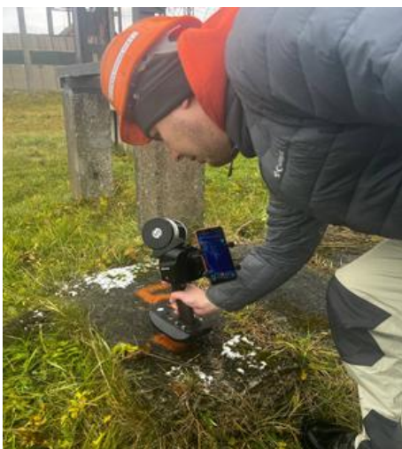
Fig. 5. Capturing the point with a scanner
