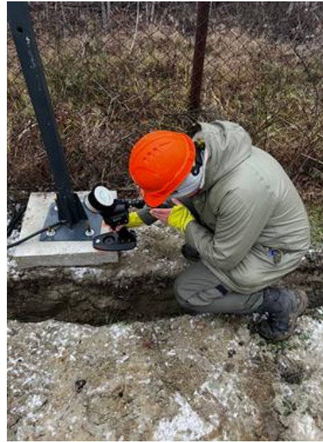
Fig. 6. Setting up the scanner on the control point
