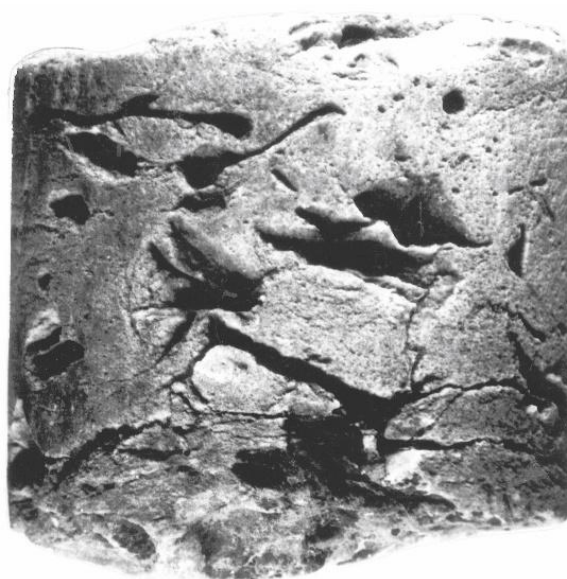
Fig. 6. Photo of oil-saturated sandstone core from well 1-Kampanska (interval 4,640-4,657 m).
