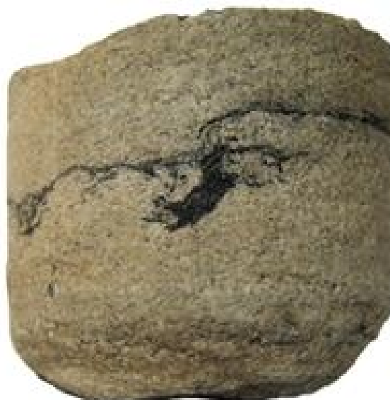
Fig. 5. Photo of the core with cavities and cracks from well 17-Semyrenkivska.
