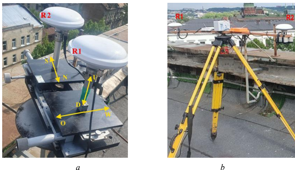
Fig. 7. Devices used for testing the developed GNSS receiver in static and kinematic modes
