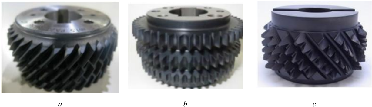
Fig.10. Conical skiving cutters with helical teeth (a) and straight teeth (b) and cylindrical skiving cutters (c)
