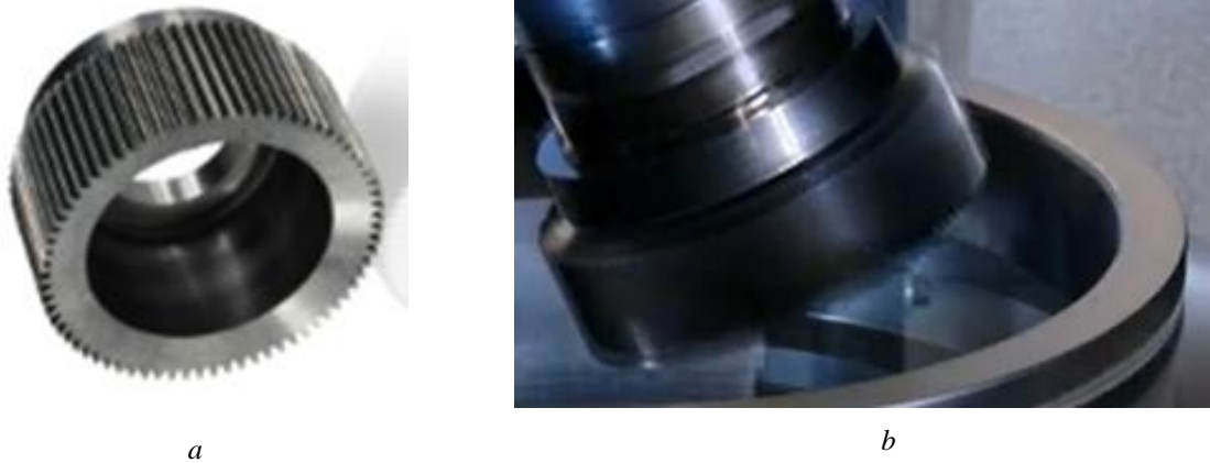
Fig.9. Spur cutter (a) and machining of a helical gear (b)
