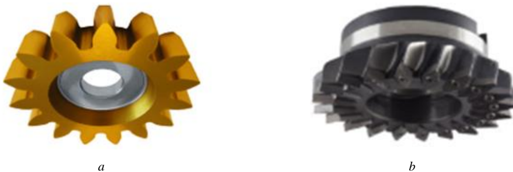
Fig.8. Conical and cylindrical solid disk-type skiving cutters
