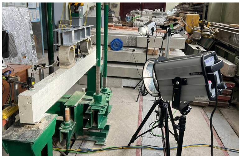
Fig. 5. General view of the reinforced concrete beam from the side of the Digital Image Correlation.
