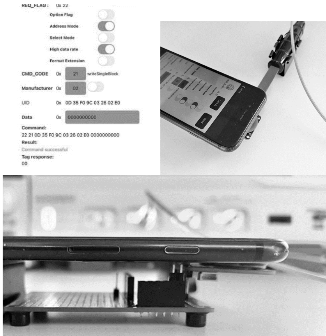
Fig. 7. “Write single block” command waveform capture setup
