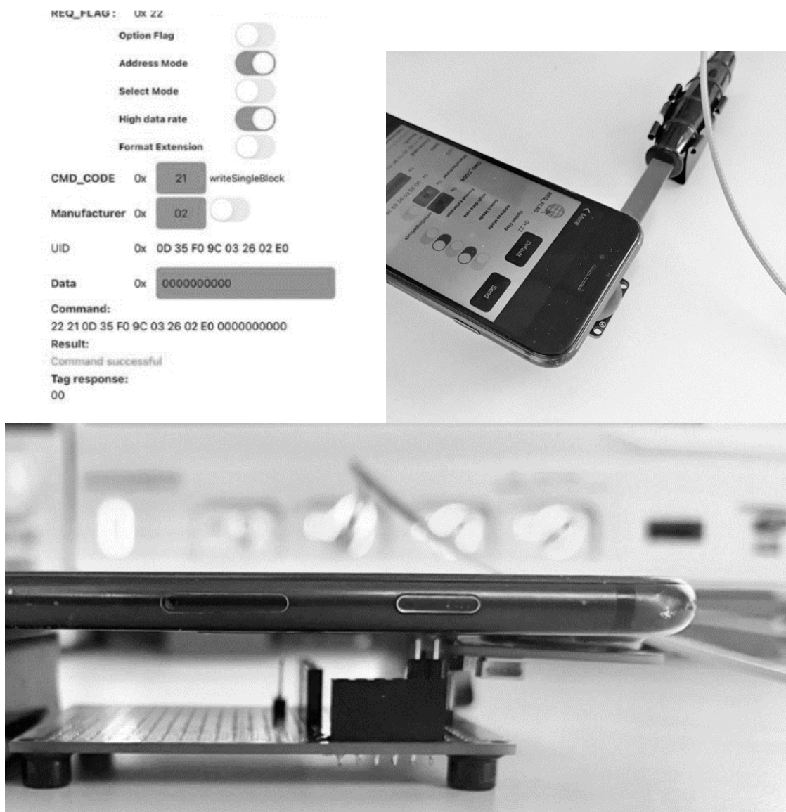
Fig. 7. “Write single block” command waveform capture setup
