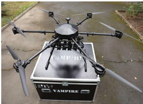
Fig. 2. Multirotor unmanned aerial vehicle 'Vampire' (Multirotor UAV) [44]
